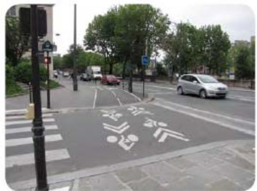
Pavement markings indicate travel direction at a minor roadway crossing on this cycle track in Paris, France.
