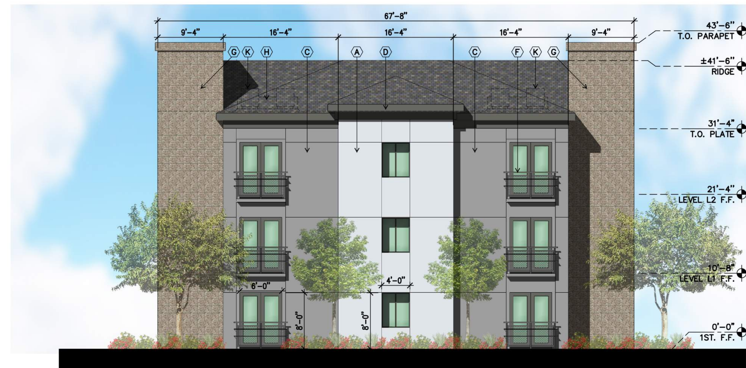
BLDG. TYPE 1 FRONT ELEVATION
