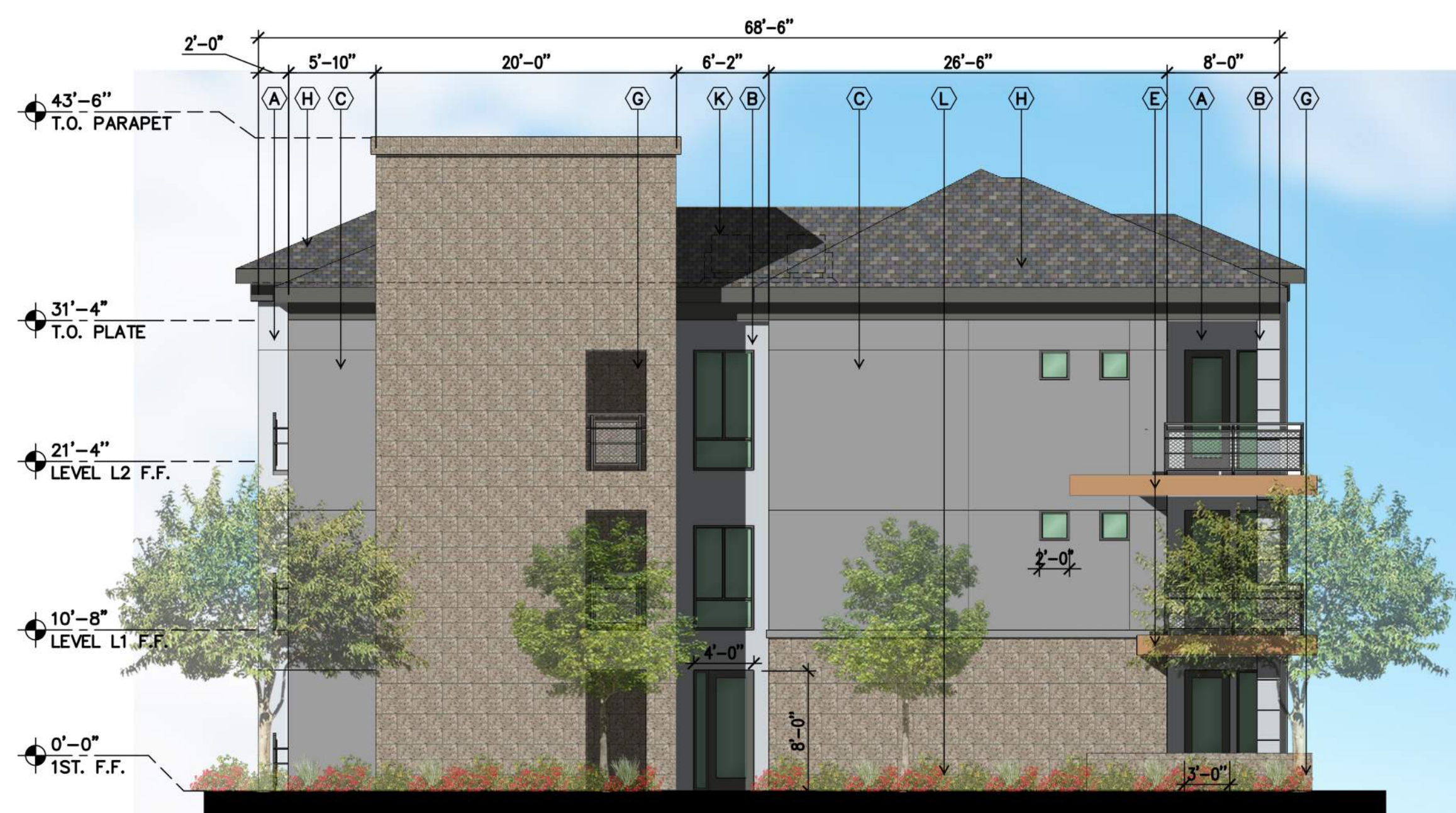
BLDG. TYPE 1 RIGHT ELEVATION
