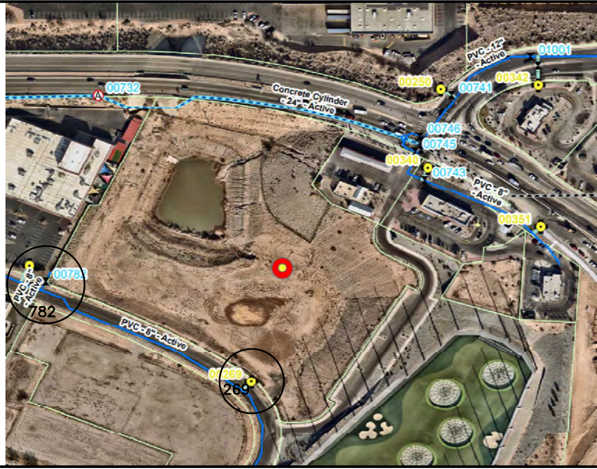
WATER SHUT-OFF PLAN SHUT OFF VALVES # 782 AND #269
