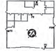
FIRE EXTINGUISHER LOCATION AT THE NEW HANGAR @ DOUBLE EAGLE II AIRPORT ADDRESS: 7401 PASSEO DML VOLCAN N.W. ALBUQUERQUE, N.M.
