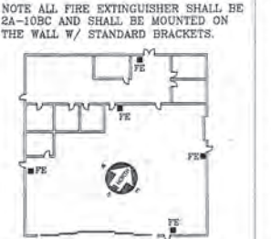
FIRE EXTINGUISHER LOCATION AT THE NEW HANGAR @ DOUBLE EAGLE II AIRPORT ADDRESS: 7401 PASEO DEL VOLCAN N.W. ALBUQUERQUE, N.M. FIRE EXTINGUISHER LOCATION DETAIL NO SCALE
