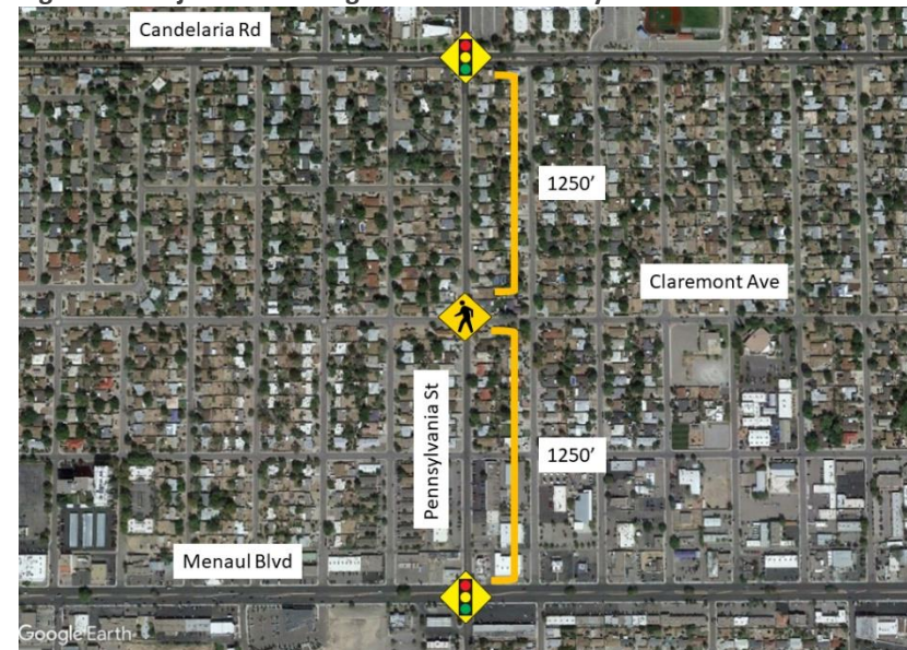
Figure 54: Adjacent Crossing Locations at Pennsylvania St
