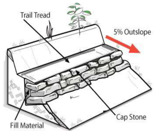
Figure 6: Typical MPOS Design for Natural Retaining Walls
