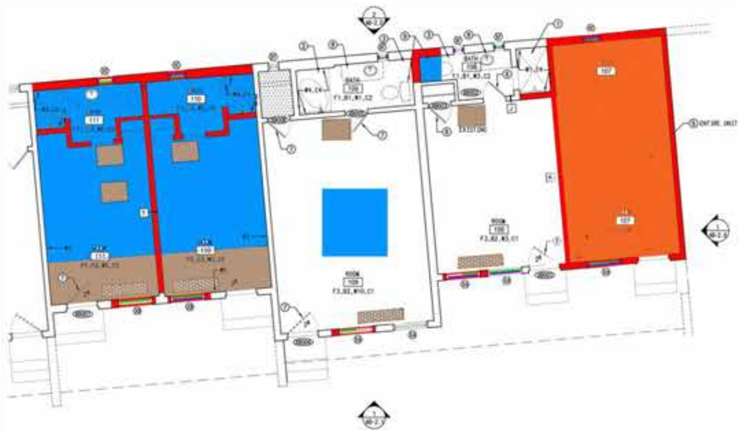
EXISTING/DEMOLITION FLOOR PLAN - BUILDING B - SOUTH
