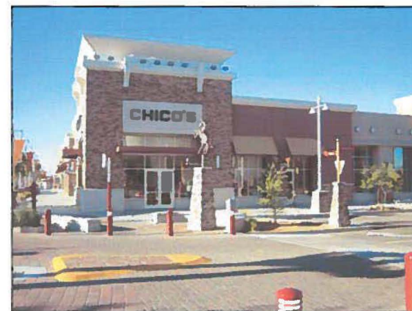
Distinguish pedestrian surfaces from driving surfaces to enhance pedestrian activity and attractiveness of walkways.
