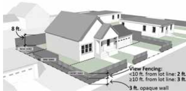
Residential View Fencing (Requires Variance – ZHE)
