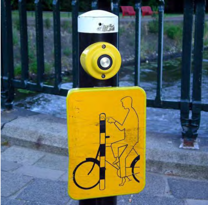
Example of curbside bike button.
