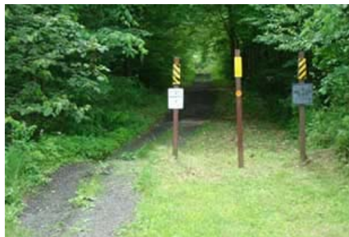
Photo of bollards on the Delaware and Hudson Rail Trail in Pawlet VT. Trail users created a new trail to get around the bollards.
