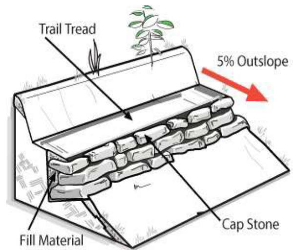
Figure 6: Typical MPOS Design for Natural Retaining Walls
