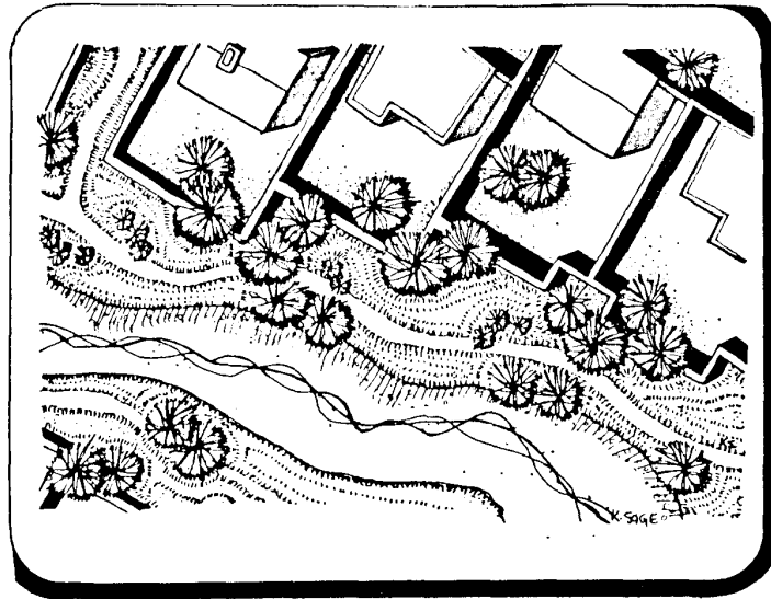
STAGGERED PERIMETER WALLS.
