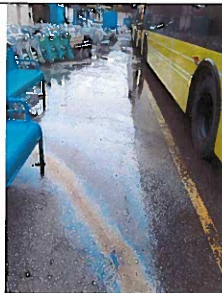
Oil sheen observed near bus parking on south side of Yale Transit Facility near outfall Y1.
