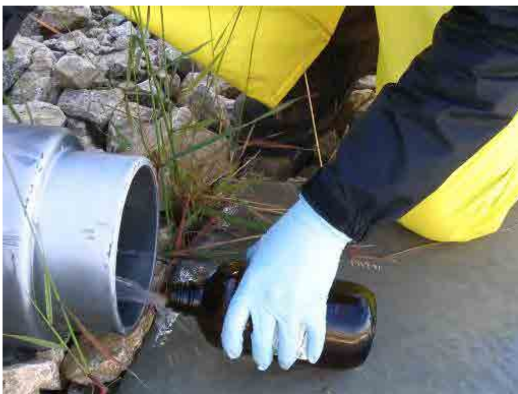
A stormwater grab sample is collected directly into the sample container.
