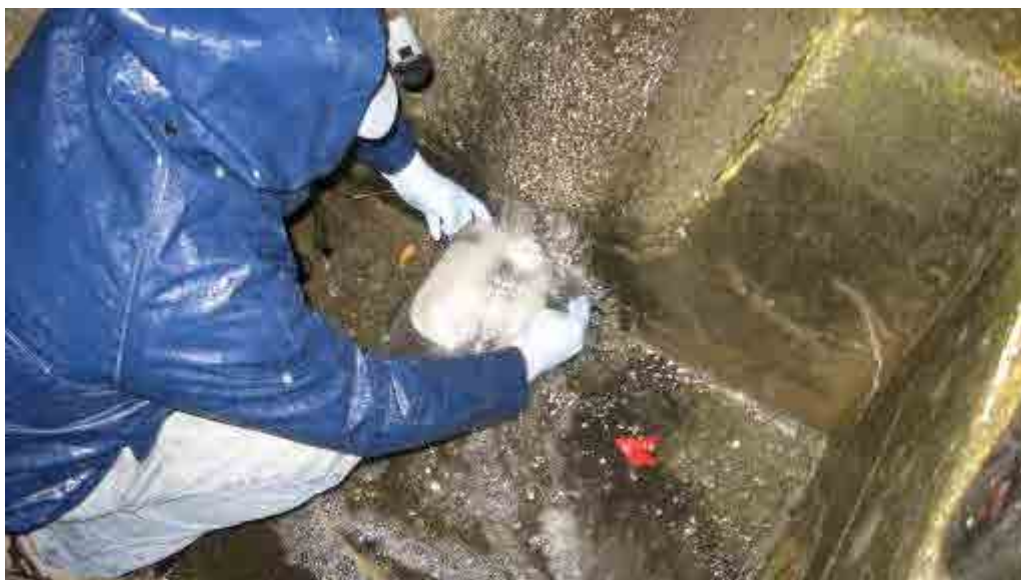
Collecting a sheet flow stormwater sample.
