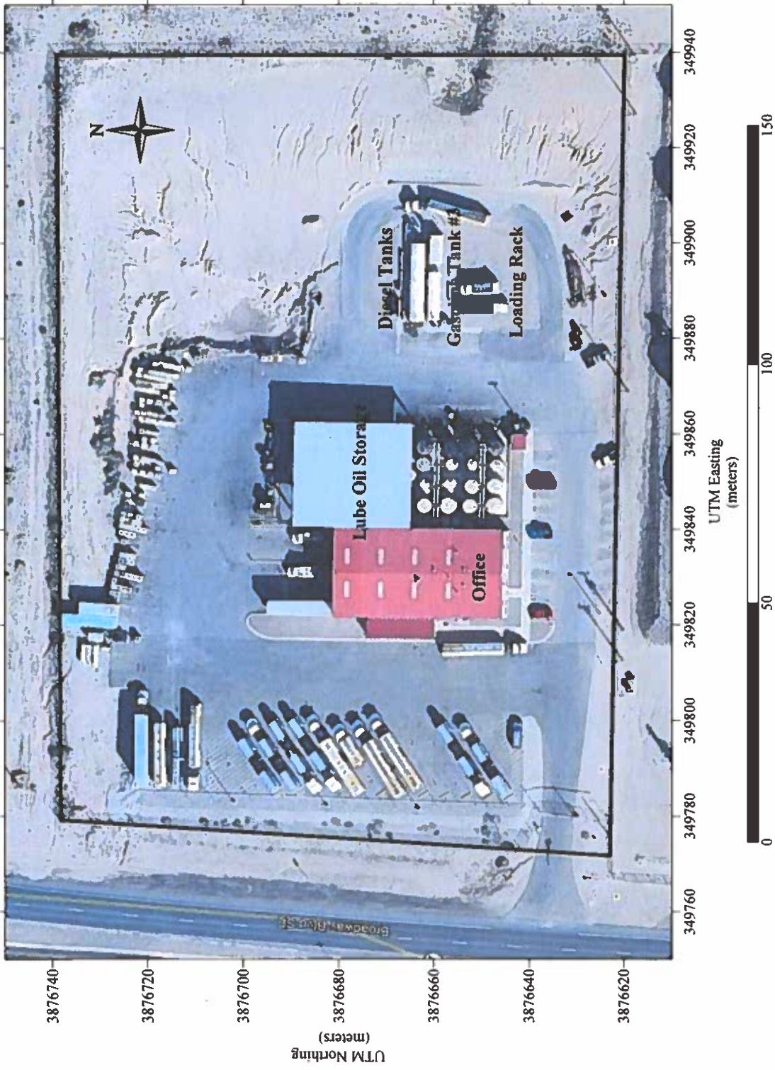
Figure A-1: Honstein Oil's Broadway Plant Layout
