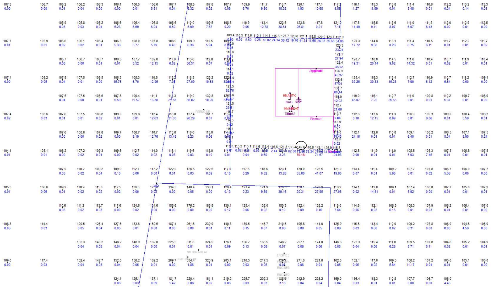
Figure 5. 1-hour NO 2 model MAXDCONT Viewer results – Star Paving contribution is lower value, background included in total upper value.
