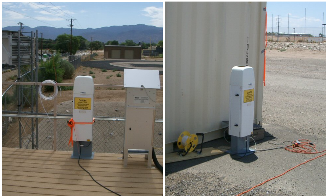
Figure 1-15. Ceilometer located on the roof of the Del Norte site (left) and at the Balloon Fiesta site (right)
