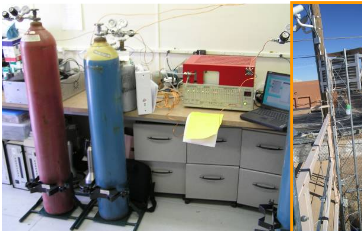
Figure 1-4 Photograph of the online GC system at the Del Norte site and the sampling inlet (left insert)
