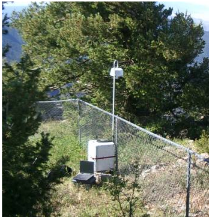
Figure 1-14 Environmental enclosure of the 202 O 3 Monitor
