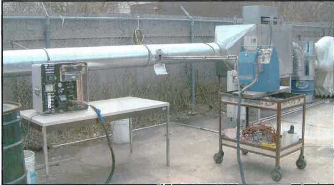
Figure 1c: PM Emissions Monitoring in Progress Using Stack Testing Equipment
