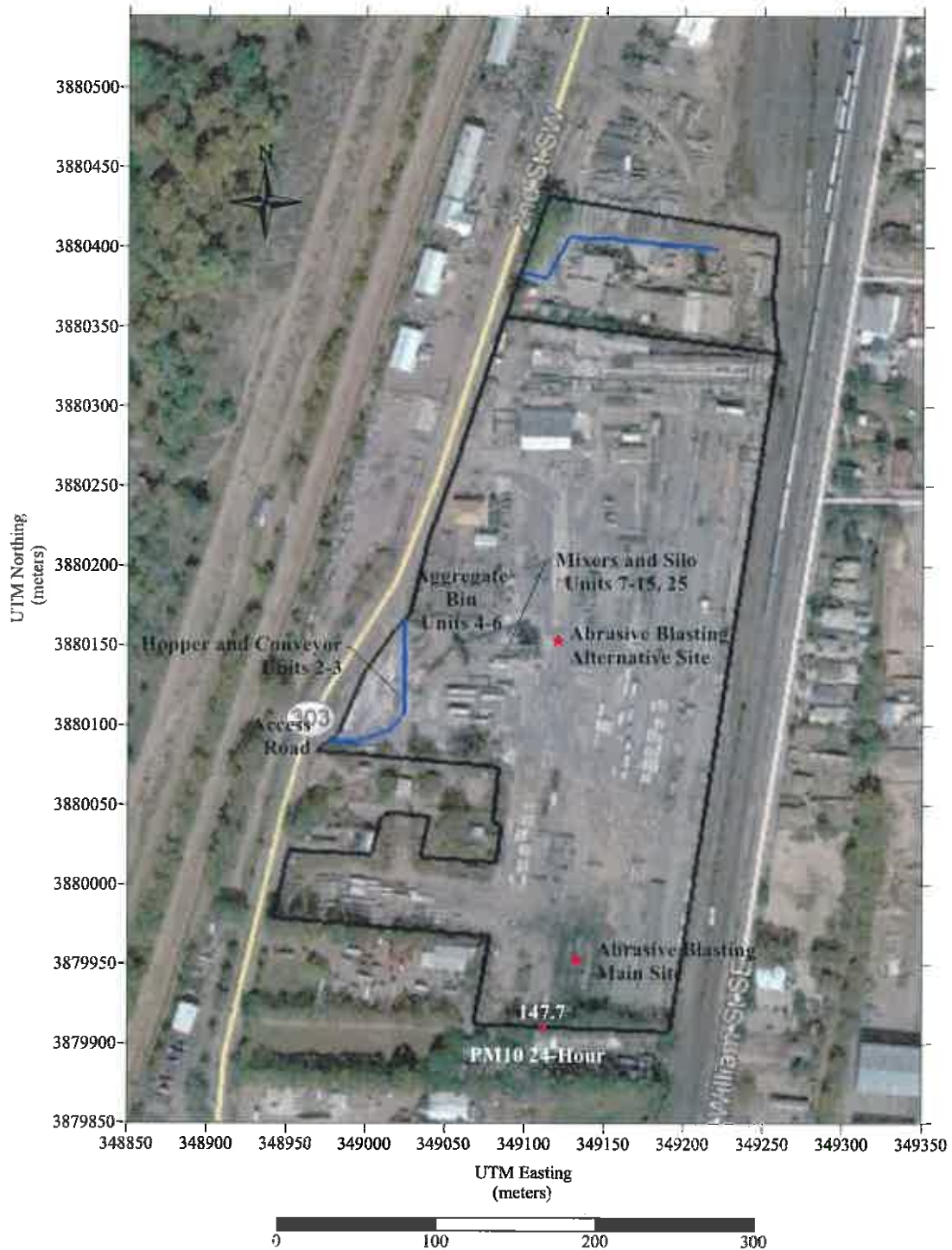
Figure 4: Aerial Map Showing the Location of the PM 10 Highest 2 nd High 24-Hour Model Results ( \mu\text{g}/\text{m}^3 )
