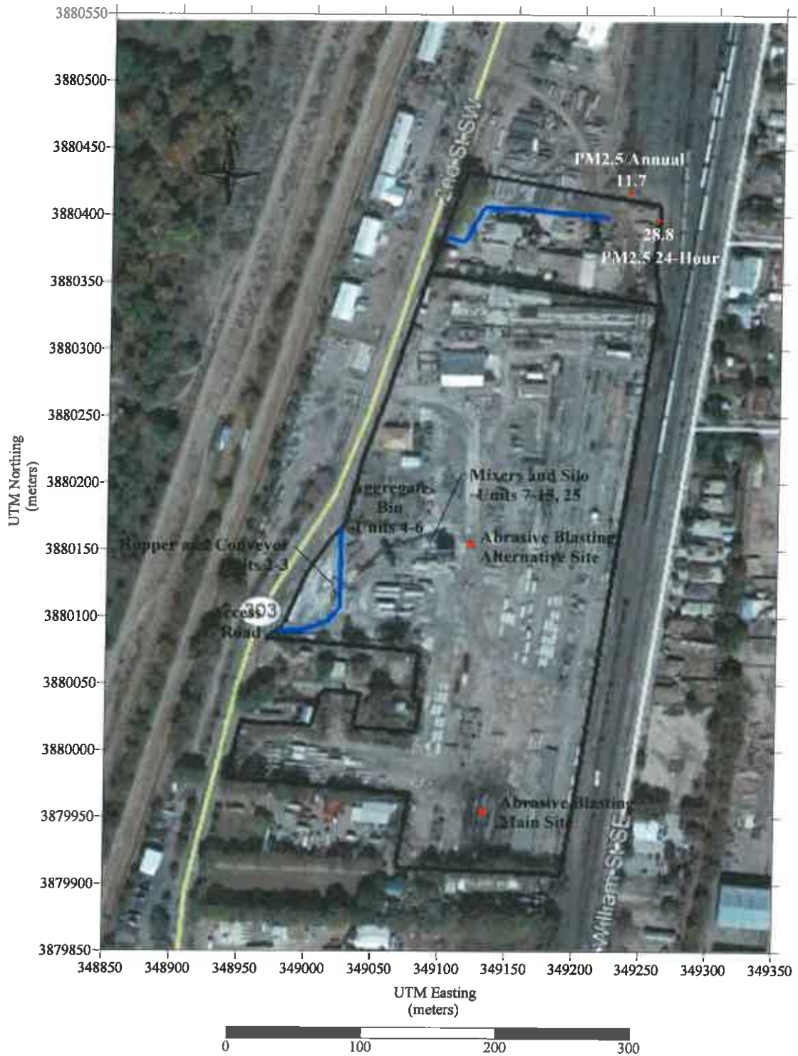
Figure 3: Aerial Map Showing the Location of the PM 2.5 Highest Model Results ( \mu\text{g}/\text{m}^3 )
