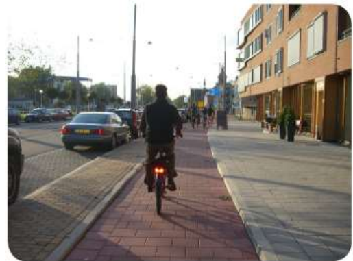
Cycle track with curb separation, Amsterdam.
