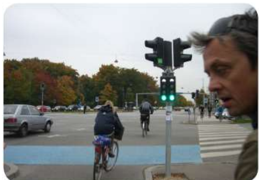
Bike-specific signals are small and placed on the near-side of traffic.
