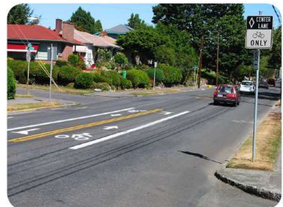
Example of a bicycle left-turn pocket.
