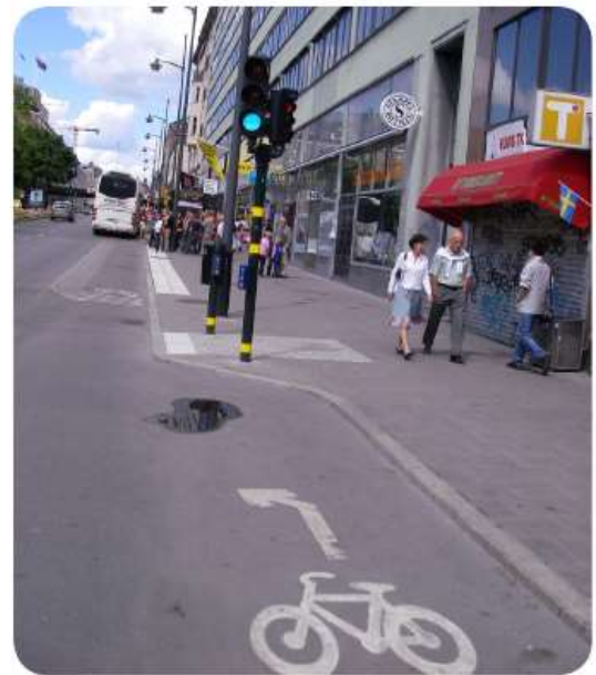
Left-turn from a cycle track on the right via bicycle-signal phase in Stockholm, Sweden.
