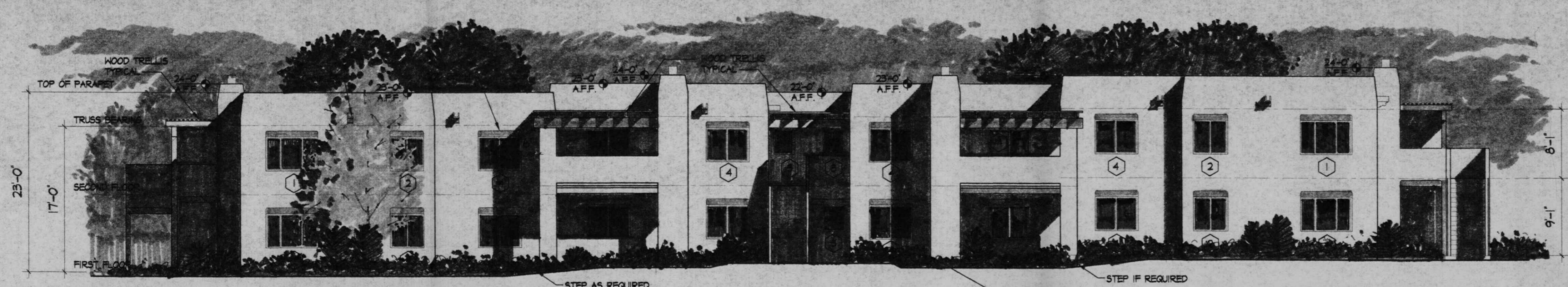
16-PLEX BUILDING FRONT ELEVATION (REAR ELEVATION SIM.)
