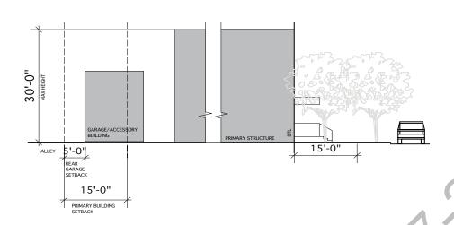
Figure 29: Level 4 Building Section
