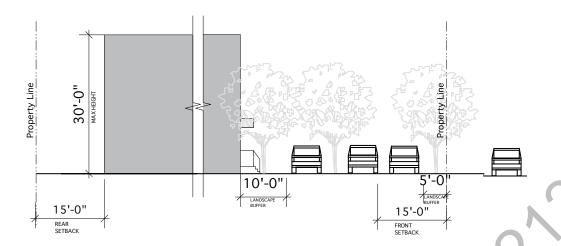
Figure 17: RMF2 BUILDING SECTION DIAGRAM
