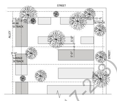
Figure 28: Level 4 Building Placement
