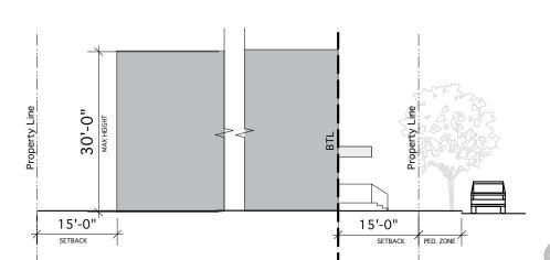
Figure 15: RMF1 BUILDING SECTION DIAGRAM
