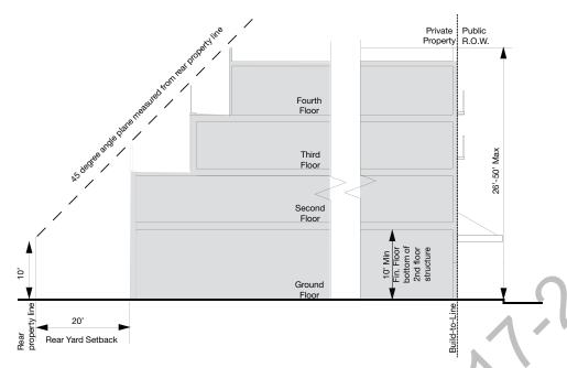
Figure 13: YCC BUILDING SECTION DIAGRAM
