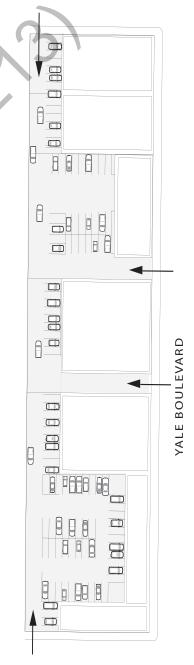
Figure 10: CONCEPTUAL PLAN SHOWING LOT ACCESS VIA SIDE DRIVE AISLES AND REAR ACCESS EASEMENT OR ALLEY.
