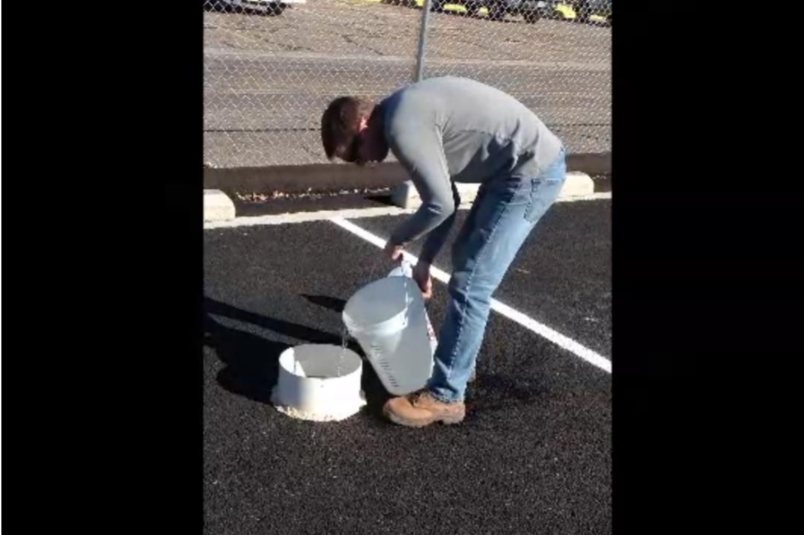
Infiltration testing of porous asphalt (ASTM Method C1701/C1701M-09)
