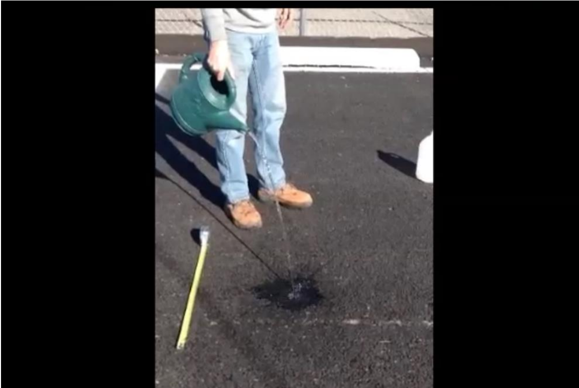
Infiltration testing of porous asphalt by "Greenbook Method"
