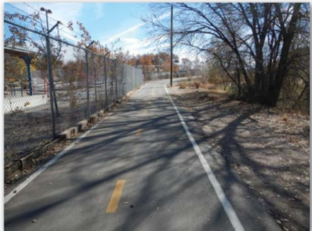
Figure 63. Segment 5, Trail narrowing by fencing, timber curb and power pole
